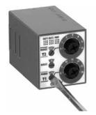
Use a flat screwdriver with a diameter of 4 mm maximum to turn Time Range Selector and gain time range as shown in the table below. Note that the selectors do not turn infinitely.
