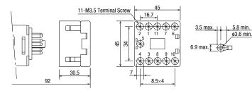
(Finger-safe 11-pin Screw Terminal Wiring Socket Adapter: SR6P-C11)
