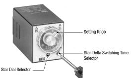
The scale range on the star side can be selected from four different ranges of 0 to 5, 0 to 10, 0 to 50, and 0 to 100 displayed in the six windows by turning the Star Dial Selector. Note that the selectors does not turn infinitely.
