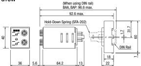
• Calculate the dimensions for mounting, referring to the diagrams of SR2P-06A on Relay Sockets catalog.
