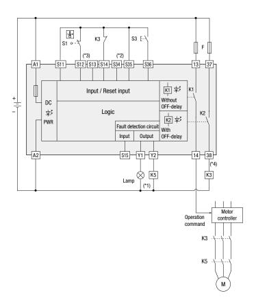
S1: Safety switch S3: Reset switch for a fault
