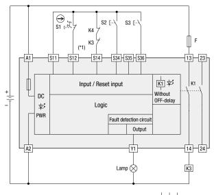
S1: Emergency stop switchS2: Reset switch for startS3: Reset switch for a fault
